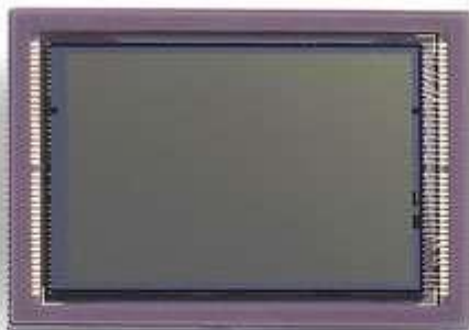
Full frame sensor (1Ds, 1Ds Mark II, 5D) 36mm x 24mm - equivalent to 35mm film
